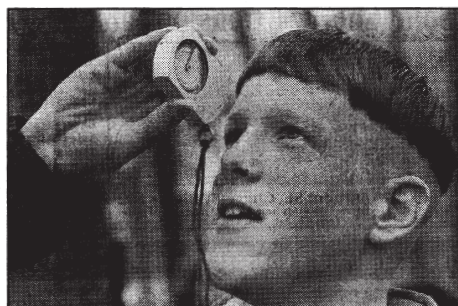
Edward Fox, 14, measures the height of a tree outside Shepherd Hill with a clinometer.
